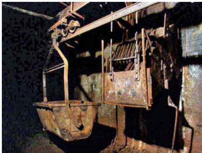
Machinery for loading ore directly onto the aerial ropeway at the bottom of the entrance incline. Photo Jochen Duceck
